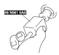
3. Raise the stopper, and pull the SST (49 N061 0A0) from the piping.
